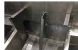
TRANSOM BRACES 5 transom braces tied to the longitudinal structure
