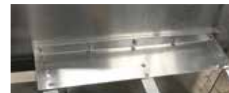
TRANSOM BRACES 5 transom braces tied to the longitudinal structure
