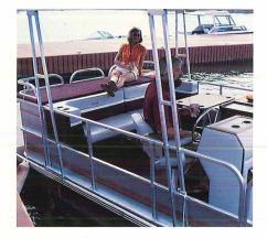
Starcraft's Stardecks come standard with the largest pontoons in the industry–19"x24"– which keep the deck surface high and dry. The deck itself is 3/4-inch Wolmanized plywood, and carries a heavy load – plus a lifetime guarantee. Among many other standards is a hard top canopy.
