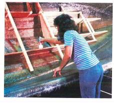
apply extra layers of woven roving. And we actually put string glass in the bottom the strakes – that means no air bubbles – and then inforce the strakes with a combination of woven roving and mat glass. Did you know that some boat companies actually fill their strakes – the main component for linear strength in the hull – with PUTTY?
