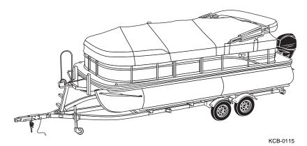
When removing the cover, grasp the material on both sides of the snap and pull it away from the boat slowly to prevent damaging the cover material. If the snaps are difficult to remove, apply a coating of paraffin wax before installing the cover again.
