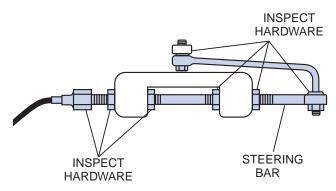
TYPICAL MECHANICAL OUTBOARD ENGINE STEERING LINK
