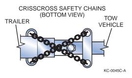
Safety chains must be rated at the same or greater weight capacity as the trailer's GVWR.
