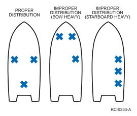
! WARNING Sinking Hazard: NEVER exceed the USCG certified maximum capacities under any circumstances. Exceeding the limitations stated on the capacity plate can cause the boat to sink or the passengers and/or operator to drown, resulting in death or serious injury.
