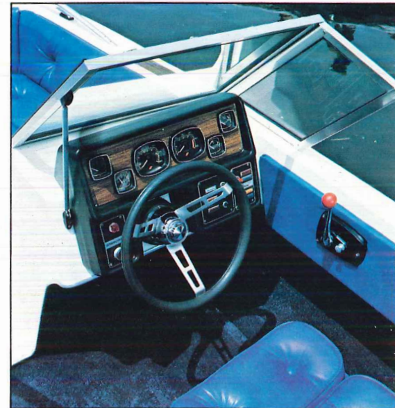
The TriStar 171/O sports a unique "modular" dashboard—that is easily removable for repairs.
