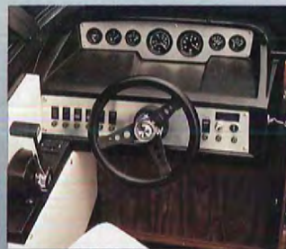
A sunshade makes reading the instruments a lot easier on bright days.
