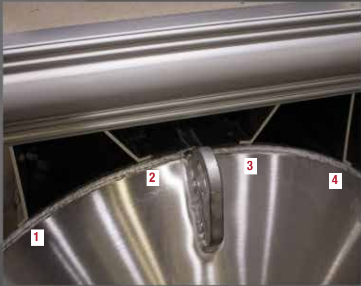
4 POINT DECK TO HULL FUSION Starcraft deck brackets have 4 points of fusion for an extended area of contact with the tube. In addition to providing increased strength and support, this reduces frame twist and racking in rough water and guards against tube fatigue.
