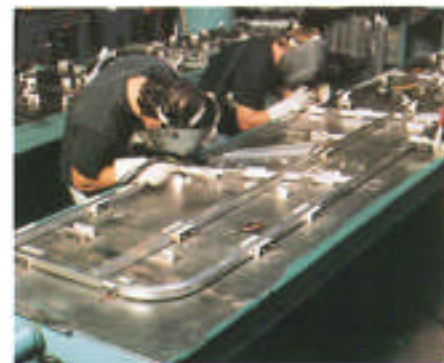
After being jig-assembled, all side fences are analyzed prior to final assembly to eliminate oxidation and discoloration.
